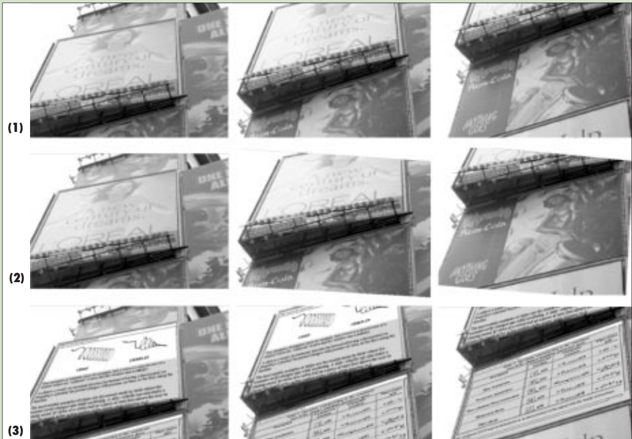
Figure A. Filtering out unwanted advertising messages: (1) Advertising can be distracting and annoying. (2) A wearable computing device together with an EyeTap system (see the other sidebar) creates a modified perception of the advertising. (3) It then replaces the advertising with subject matter useful to the user.
